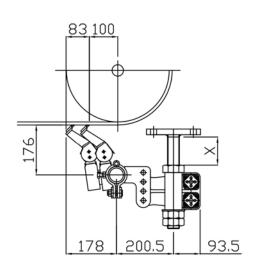
"X" = the tensile axis, the length must be at least 90 mm.
